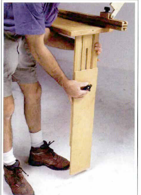
6. Height adjustment at the turn of a knob. A hardwood runner riding in a router-cut groove keeps the two parts of the legs aligned as they adjust to the desired height. A single knob locks them in position.
